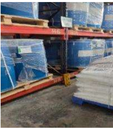
Maximum stacking height needs to be defined. SWL marking needs to be done on storage racks
