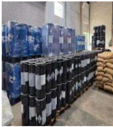
Walkways, Emergency Exits, to be kept accessible all the time. Chemical storages to be done as per compatibility of the chemicals
