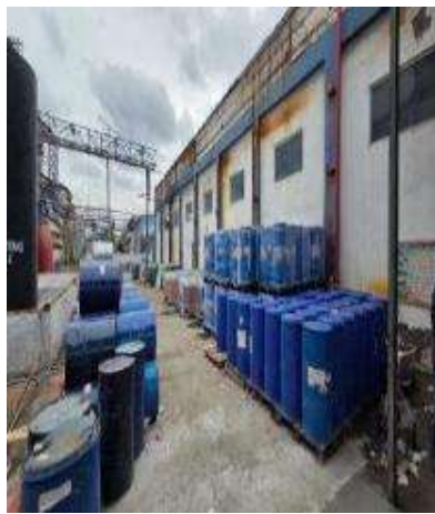
Chemical Barrels to be stored in proper place/ inside shed and away from direct sunlight
