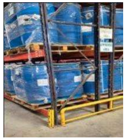
Material storage rack found bend needs to be repaired /replace
